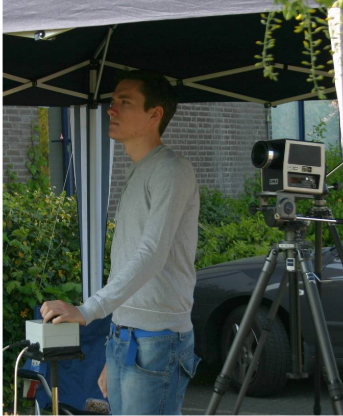
Figure 2. Subject adjusting the luminous intensity with a rotary knob. Right: light meter for measuring the surrounding luminance and the luminous intensity of the traffic lights.
