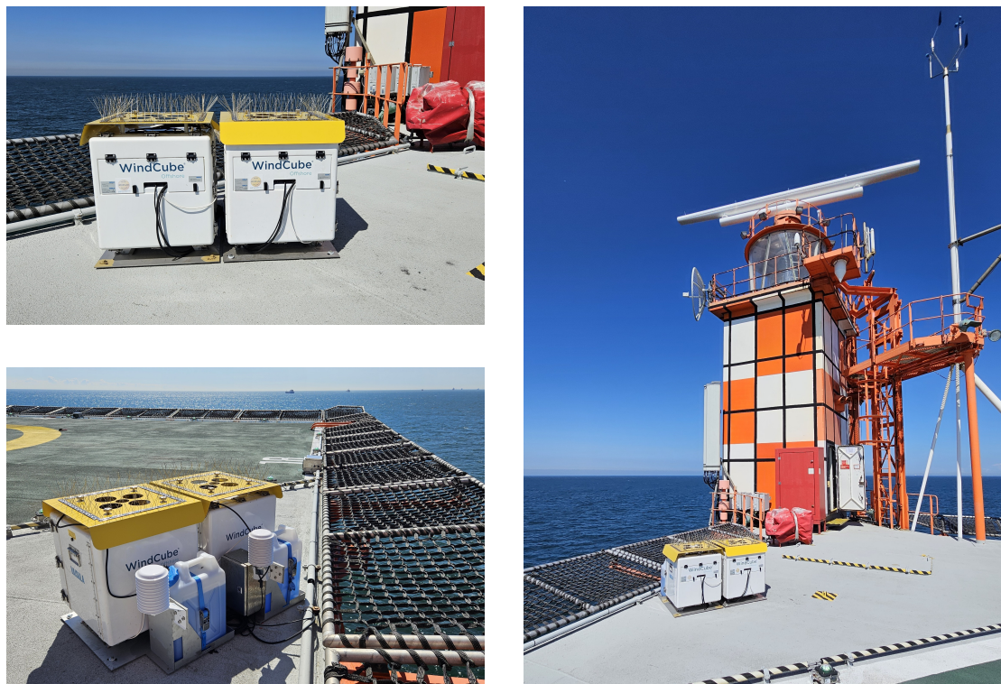
Figure 3.2: Measurement setup of two WindCube V2.1 lidars at LEG.
