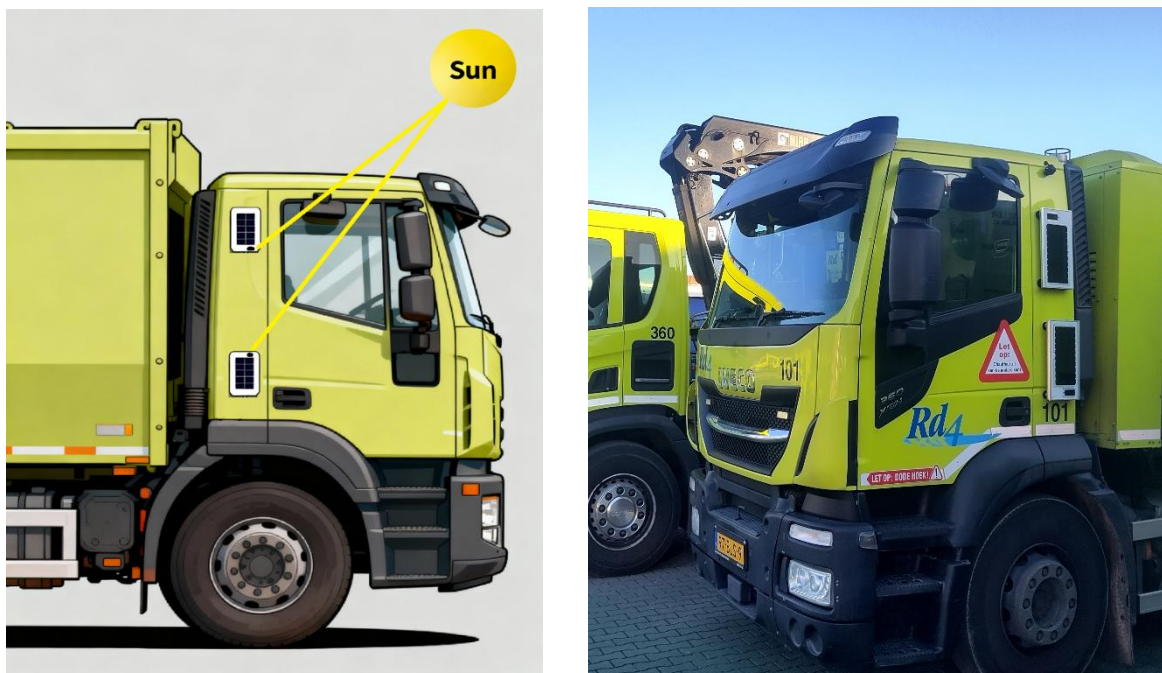
Figure 136: Schematic picture (left) and photo (right) of the sensor location on the DAF garbage truck
