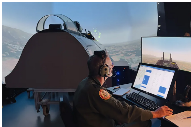
Fig. 1. The experimental set-up of the fixed-based F-16 cockpit, its projection dome, with a subject (left) and experiment leader sitting at the control station (right).
