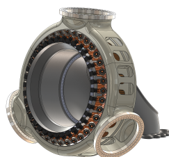
Figure 1. Schematic illustration of the OptiGen drivetrain concept with wheel–rail support system and reduced air-gap dependency on generator diameter.
