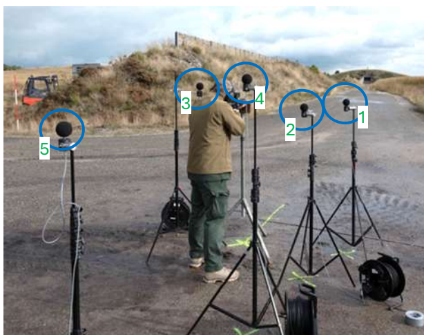
Figure 3. Outdoor measurement set-up using 5 microphones.
