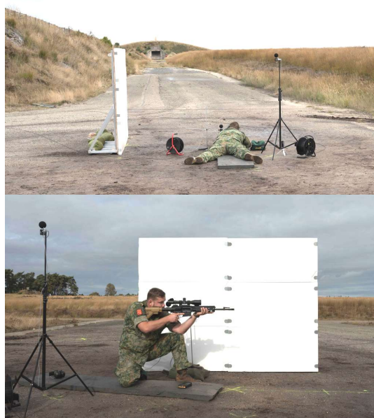
Figure 11. Absorbing screen at 2m distance (upper) and at 1m distance (lower).
