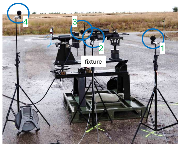
Figure 4. Outdoor measurement using a weapon fixture.
