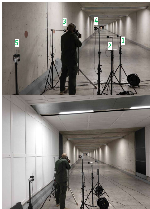
Figure 2. Measurement set-up using 5 microphones close to hard walls (upper) and absorbing walls & ceiling (lower).
