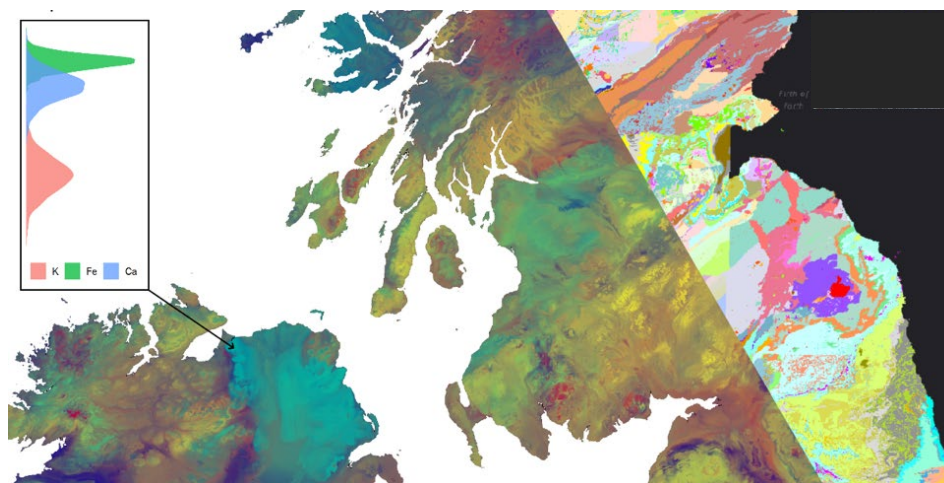
Figure 1- Left of diagonal: Bayesian deep-learned predictive map of geological properties, in this case chemical composition with a ternary colour scheme (K - red, Fe - green, Ca - blue). Posterior predictive distributions can be obtained for any location. From https://geoscientist.online/sections/features/geological-mapping-in-the-age-of-artificial-intelligence/ Right of diagonal: Traditional classified geological map, in this case British Geological Survey Bedrock Geology. From https://geologyviewer.bgs.ac.uk
