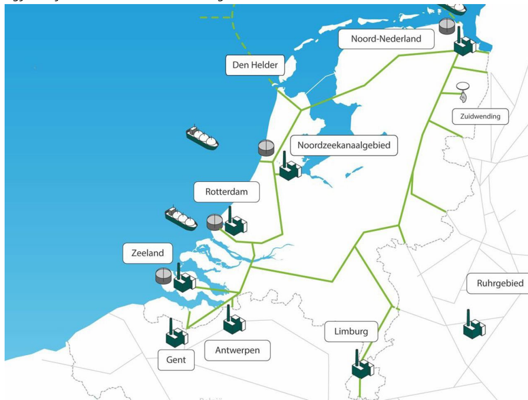
Figure 3: The hydrogen backbone connecting chemical clusters in the Netherlands, Belgium and Germany
