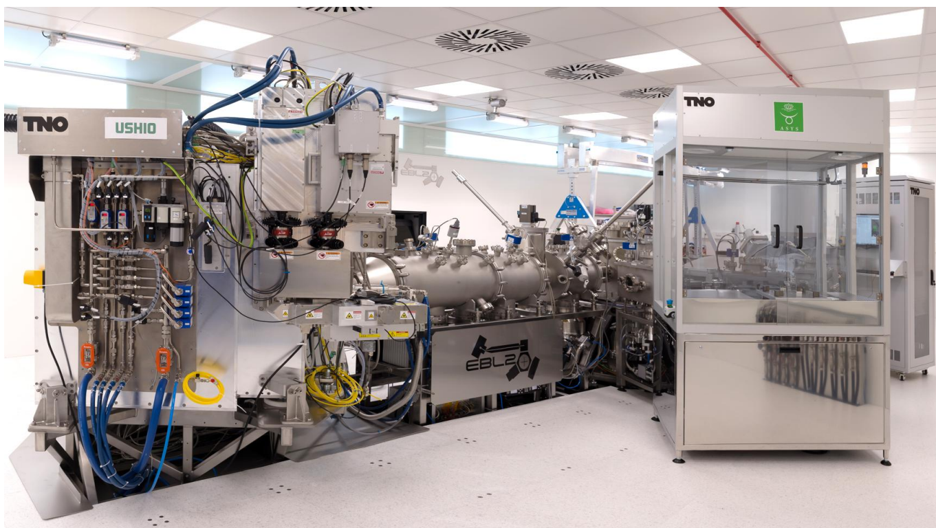
Photo illustrating the overall view of the EBL-2 research facility at TNO (left side: EUV source, center: beamline; right: sample loading module)
