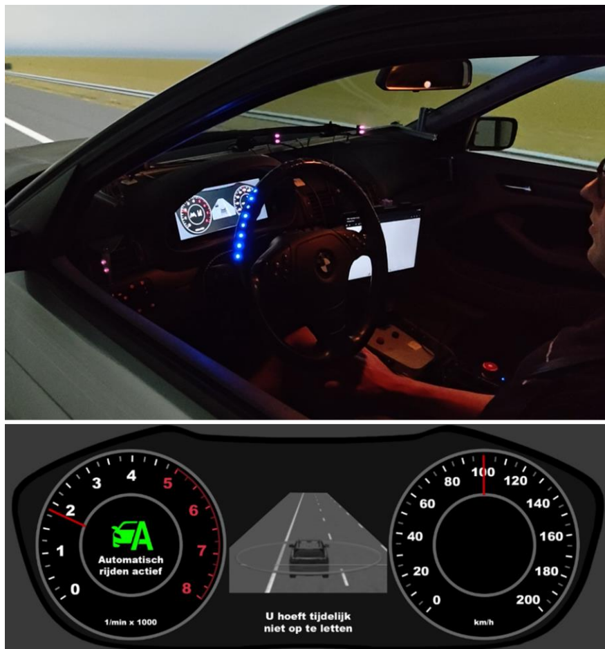
Figure 2. Experimental setup with an example of a good quality HMI designs in terms of clarity and unambiguity.
