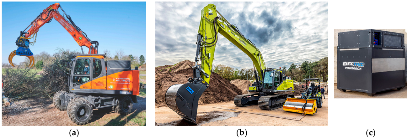
Figure 1. (a) 17-ton mobile excavator (type DX165W); (b) 35-ton tracked excavator (type DX355LC); (c) 114 kWh powerbox.
