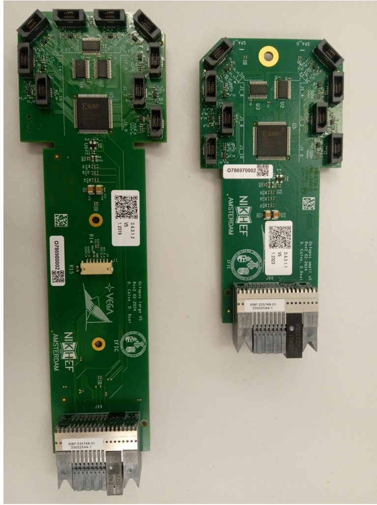
Figure 2: Set of Signal Collection Boards of the latest version.
