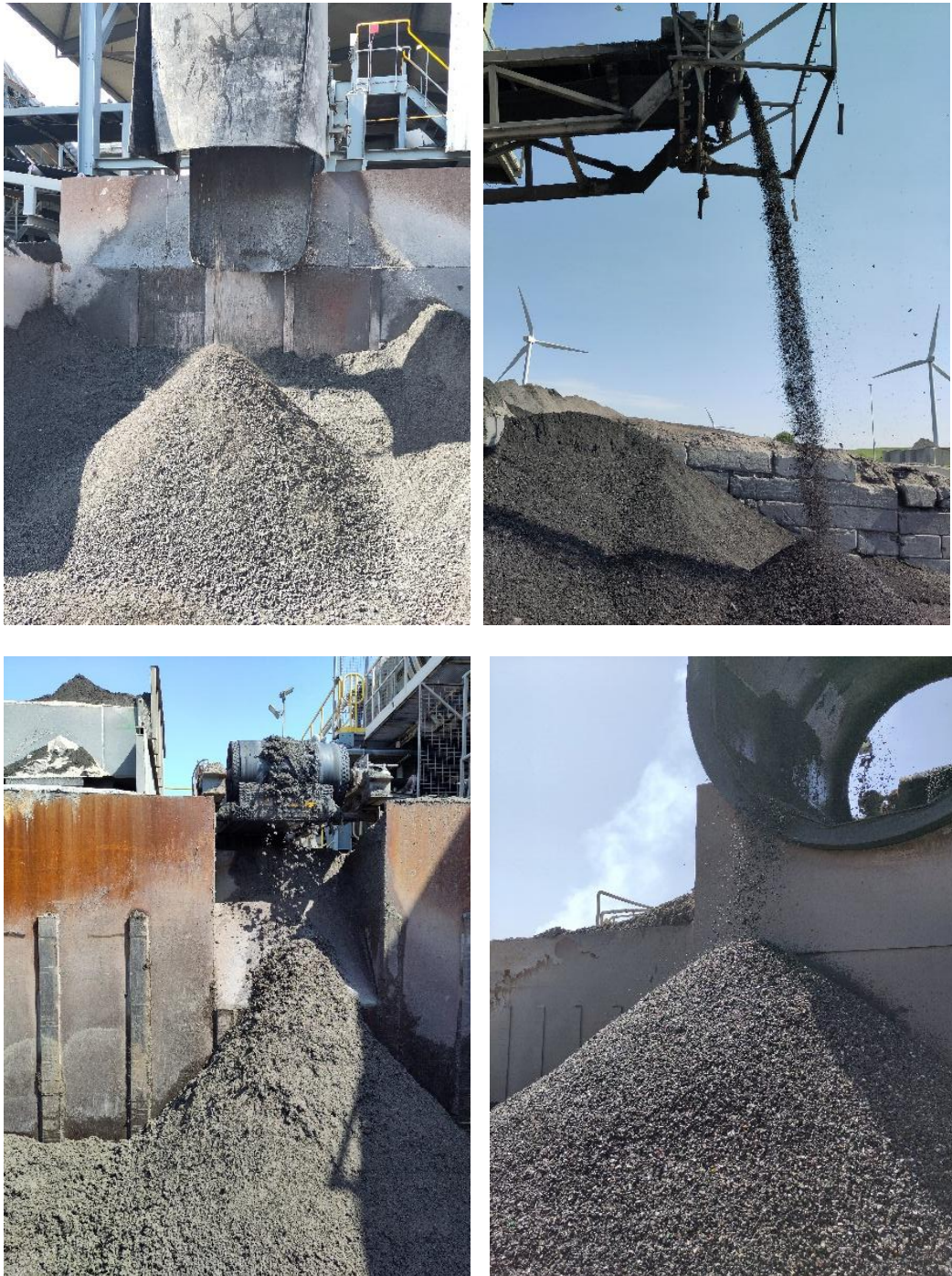
Figure 2: A photo impression of recycling steps at Heros. In clockwise rotation: ferrous slag recovery (sample W ), the medium fine bottom ash output (sample X ), washed sand (sample P ) and coarse washed concentrate (sample U )
