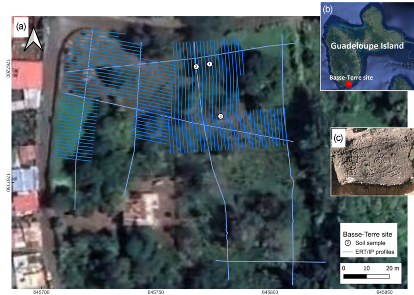
Figure 21. Presentation of the test site. (a) Test site. The lines correspond to the induced polarization profiles made in the survey. The three circles correspond to the position of the three soil samples collected in the field. (b) Position of the field data in Guadeloupe Island. (c) The site is characterized by the presence of some buried boulders, some of which are of archaeological significance (pre-Columbian rock engravings). Nowadays, the investigated area is used mostly for Creole garden-type subsistence farming, with extensive banana growing areas.
