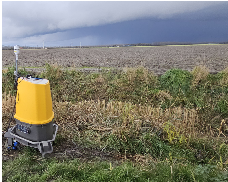
Figure 2.6: ZX300M ZX6482 lidar at the RSD verification location
