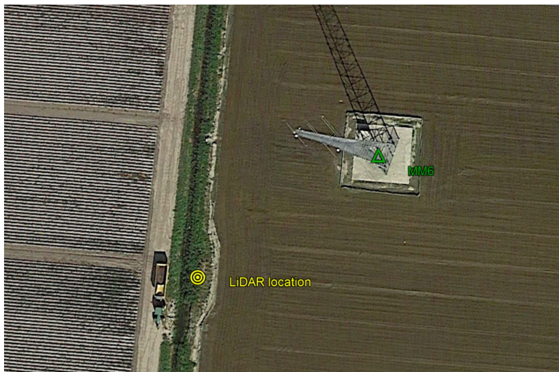
Figure 2.4: Position of the lidar at 49 m from the meteorological mast; indicated in green is meteorological mast MM6 and in yellow the verification platform
