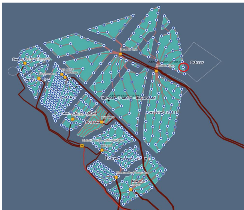
Figure 2-2: Selected scanning lidar location at the easternmost wind turbine BF5 of Borssele 1&2, indicated by a red circle (source: 4C Offshore).
