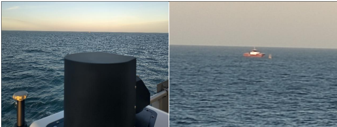
Figure 2-6: Confirmation of the heading of floating lidar system FL-West. Left: looking over the Galion scanning head towards FL-West and the CTV in the background. Right: zoomed in on FL-West and CTV.
