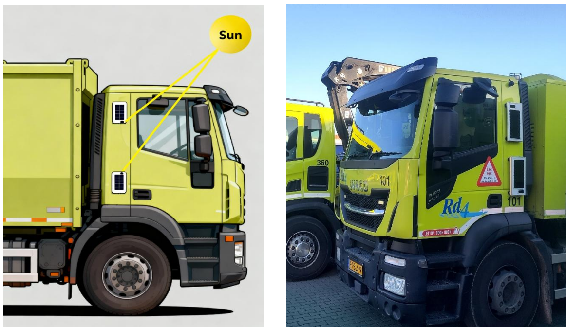
Figure 139: Schematic picture (left) and photo (right) of the sensor location on the DAF garbage truck
