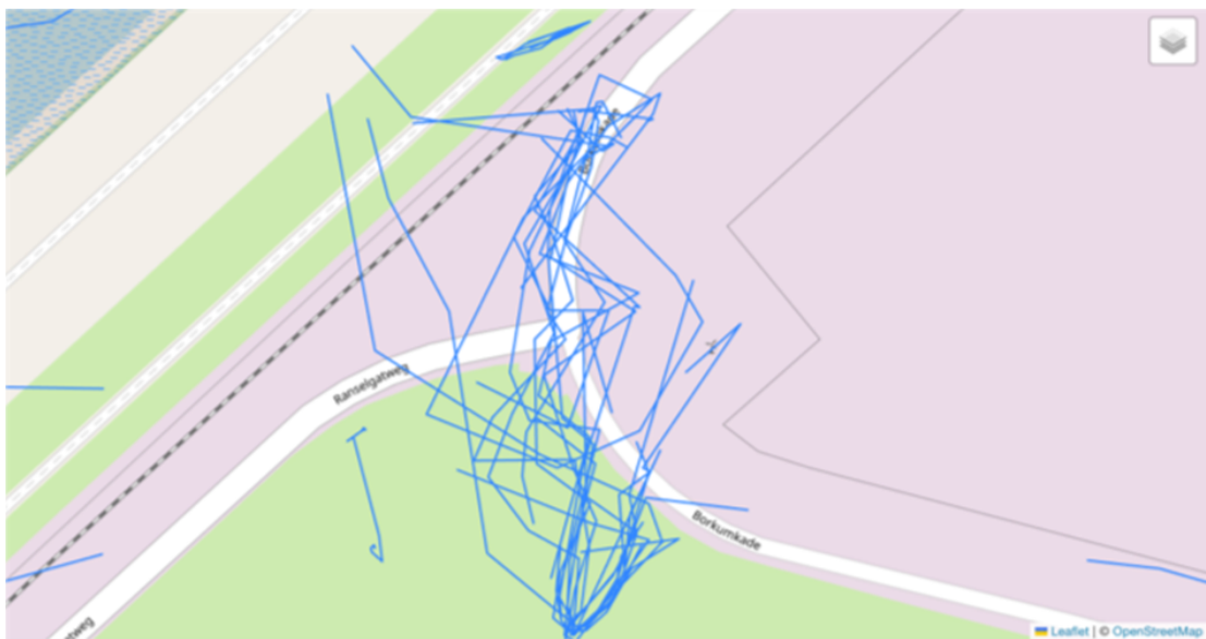
Figure 3.26: Radar tracks (mostly clutter) around the turbine 21 around the time of impact on the 10th of September 2024, map based on OpenStreetMap
