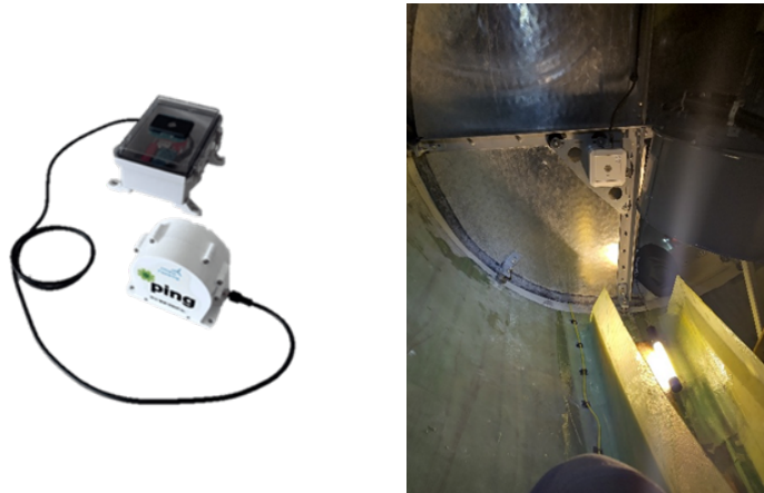
Figure 3.33: Picture of in blade microphone of Eologix-Ping and picture of the microphone installed in the blade of the turbine. Left picture by Eologix-Ping
