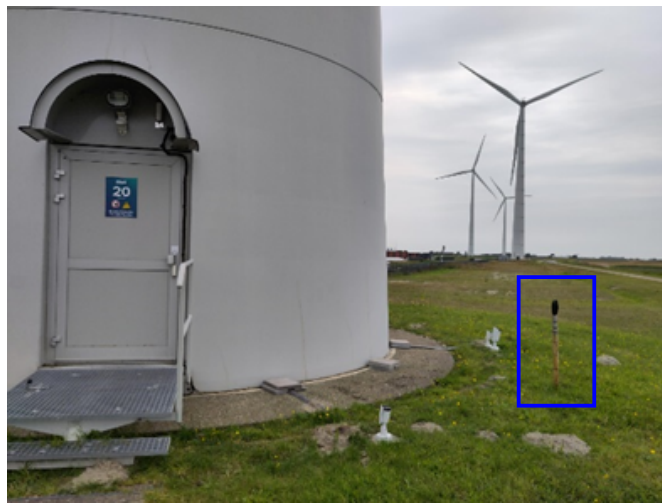
Figure 3.30: Microphone at the base of turbine 20
