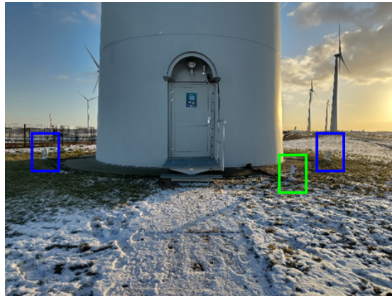
Figure 2.4: Picture of turbine 20 with two pairs of cameras on either side (in blue) plus an additional thermal camera for stereography tests (in green)
