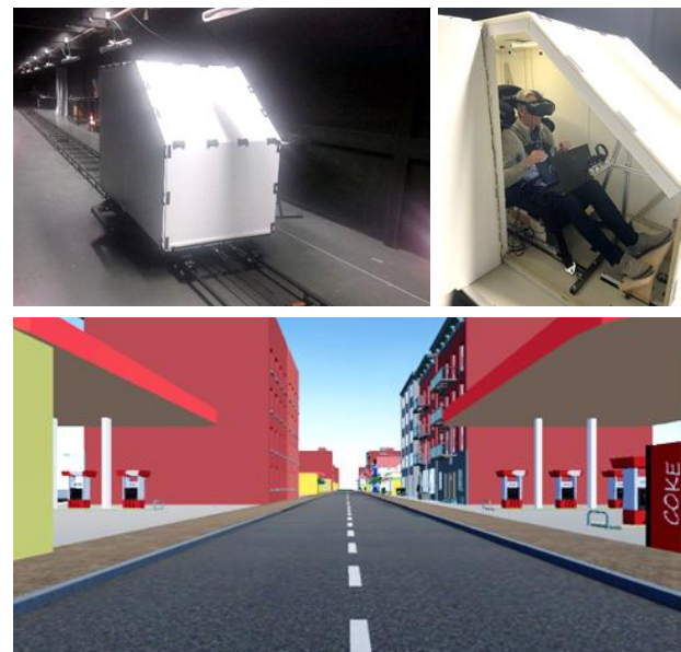
Figure 1. The 25 m linear sled (top left), the setup of the interior of the cabin, also showing the additional controller attached to the cabin (top right), and the imagery (bottom), as used in the experiment.
