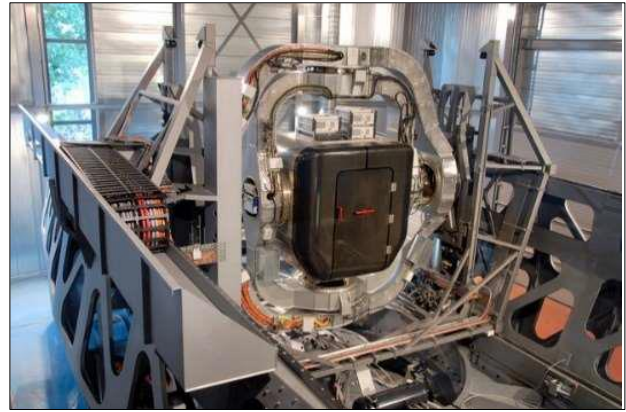
Figure 1: TNO's Desdemona facility. Although the device has six degrees of motion freedom, for the experiment described here, only the vertical degree was used
