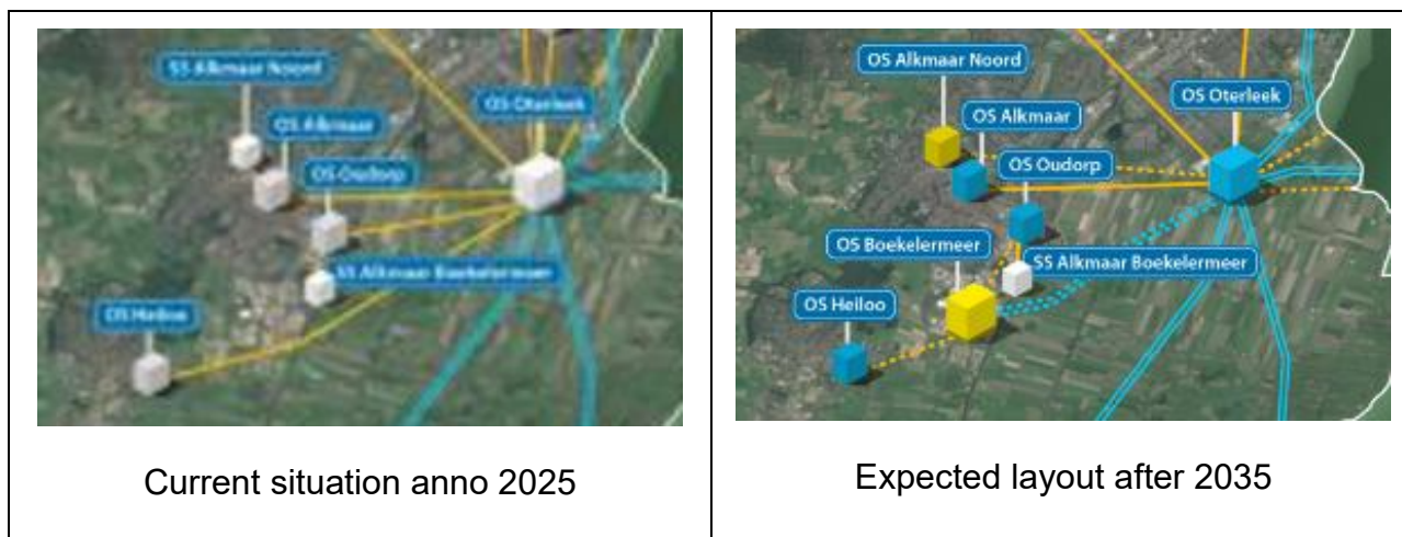
Figure 7: Electricity grid topology in the area of the FV, now (left) and after reinforcements (right)
