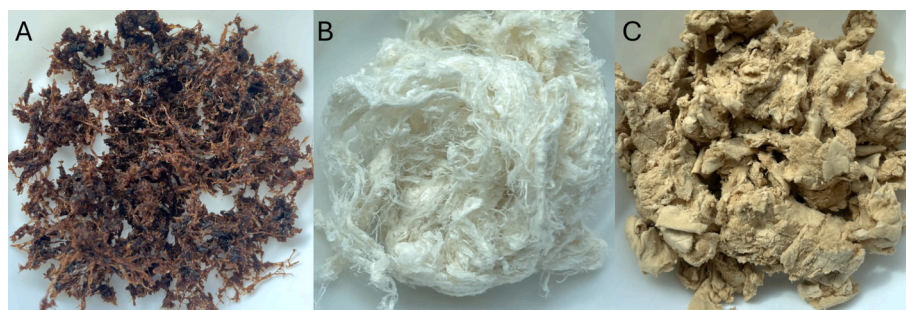
Fig. 3. (A) Photograph of the alginate extracted from the Sargassum biomass in this study, exhibiting a deep brown colour. (B) Alginate extracted from Saccharina latissima using the same extraction procedure as employed in this study, showing an almost white colour (included for visual comparison only) (C) Fucoidan extracted from Sargassum biomass, displaying a light brown colour. (For interpretation of the references to colour in this figure legend, the reader is referred to the web version of this article.)
