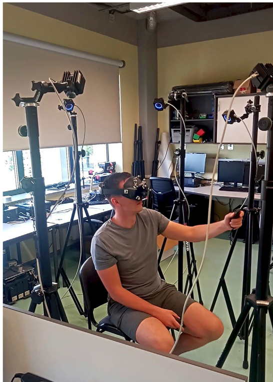
FIGURE 3 Measuring the accuracy of inside-out head tracking.
