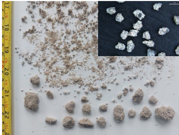
Figure 3. The main frame shows a real sample created by EPP electrodes. The smaller frame on the top right displays a microscope image of the sample within 1.4 and 2 mm size; cuttings from EPP drilling test provided by TU Dresden.
