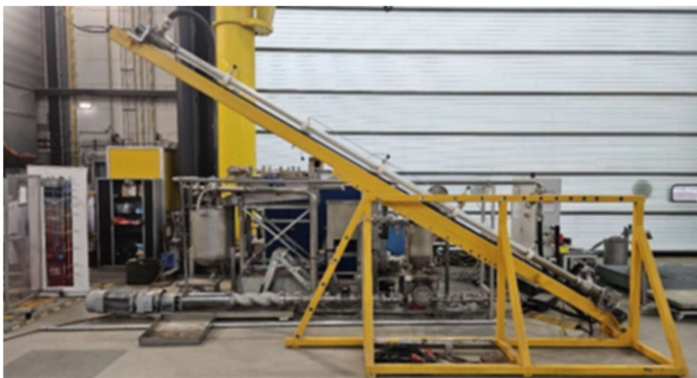
Figure 1. Cuttings flow loop at TNO's Rijswijk Centre for Sustainable Geo-Energy used for experiments.
