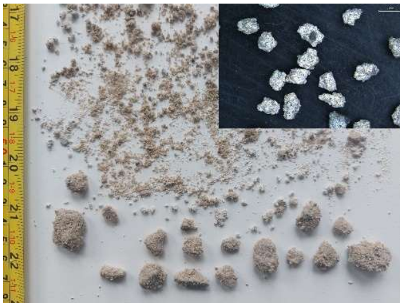
Figure 2. The main figure shows a sample of cuttings generated by EPP rock breaking, the larger cuttings being over 2 cm large. The smaller figure on the top right displays a microscope image of the sample within 1.4- and 2-mm size.
