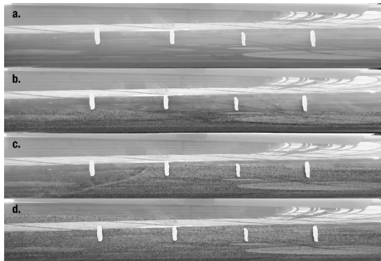
Figure 5. Four transportation regimes at 60° test section. From top to bottom: (a) free homogeneous flow, (b) dunning, (c) dynamic bed and (d) stationary bed. The distance between the white stripes is 10 cm. Flow is going from right to left.
