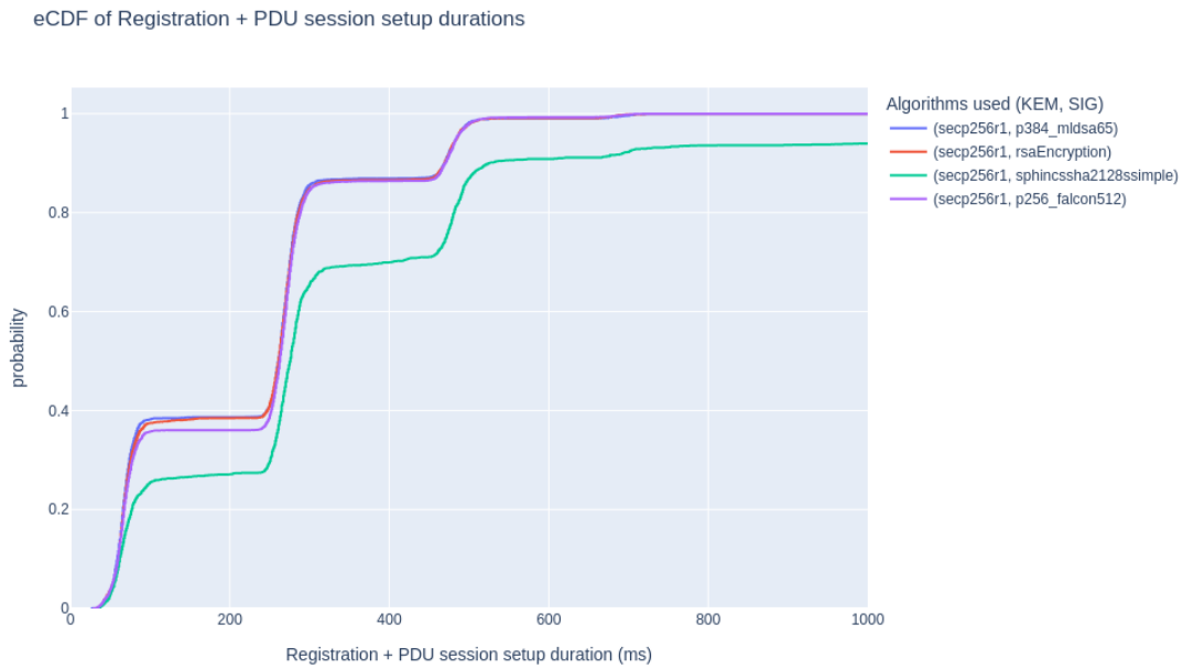
Fig. 5. Histogram showing the setup duration with various signature algorithms, combined with a conventional (ECC-based) KEM.
