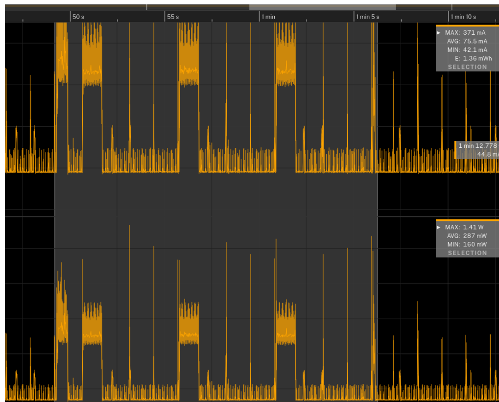
Figure 5.6: Sample of the energy consumption of the 5G modem
