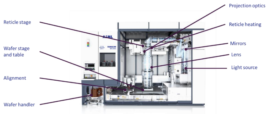
Figure 11. A TWINSKAN system and its subsystems.
