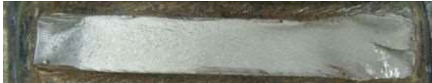
Figure 3.45 – Fracture surface of an as-welded specimen, stress range 90 MPa, fatigue life 3.62 \times 10^6 cycles.
