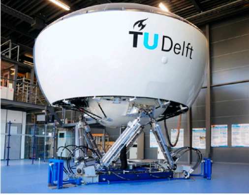
Figure 1. SIMONA Research Simulator and flight deck used in the experiment.
