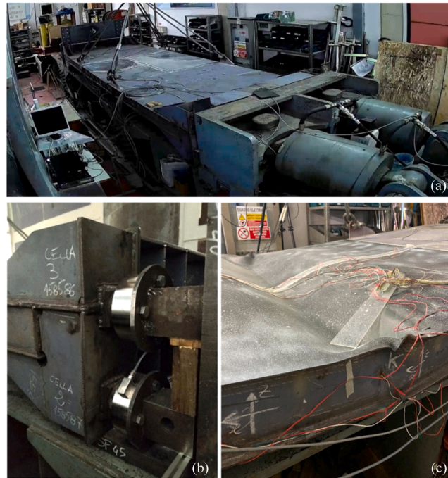
Fig. 2. (a) Top view of the specimen on the laboratory test bench. (b) System for connecting the specimen to the bench on the unloaded side through the load cells. (c) Collapsed specimen section.
