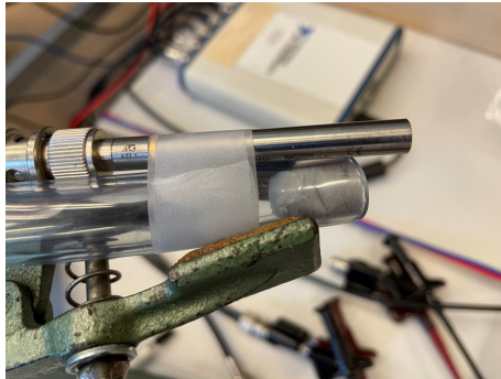
Figure 6.10: Primary source enclosure design 2, with a tube connected having 1 cm thick melamine foam at its end.
