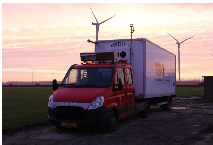
Figure 1.2: The HT8700E ammonia measurement instrument from Healthy Photon mounted on top of the truck trailer under a specially designed metal hood for rain protection.
