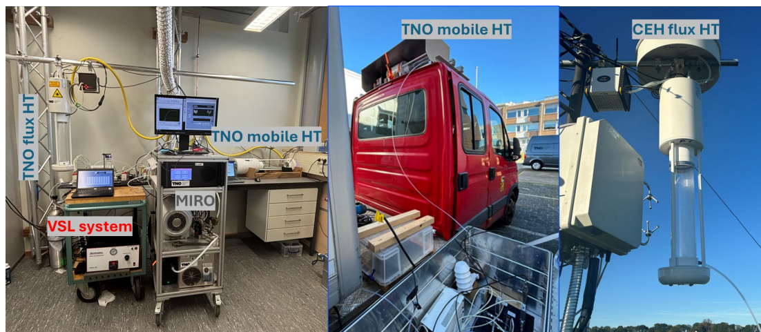
Figure 2.1: From left to right, a) VSL calibration set up at TNO laboratory to do indoor calibration of TNO mobile HT and flux HT. Note that a closed-glass cell with 3.7 L volume is applied in both HTs during the calibration period; b) VSL-TNO mobile HT outdoor calibration in TNO; c) UKCEH HT field calibration using RGM at a Dutch dairy farm during the field campaign in October 2024.
