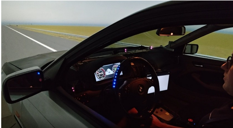
Figure 2.3 Transition phase of a scenario with flashing steering wheel LEDs.
