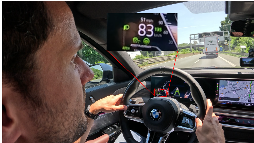
Figure 7.10: Assisted Driving Mode active and Assisted Driving Mode Plus "ready".
