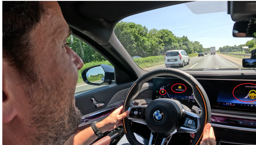
Figure 7.13: A few seconds later, Personal Pilot requests the driver to take control. The hands slightly touch the wheel, but not enough for the driver to regain full longitudinal control of the vehicle.
