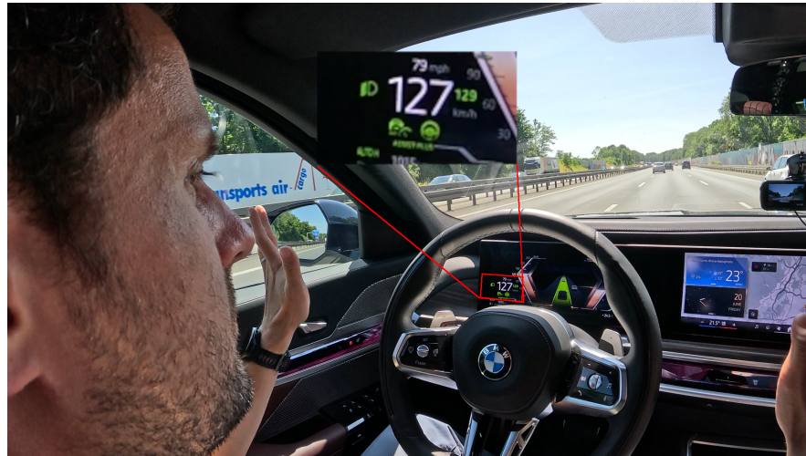
Figure 7.11: Assisted Driving Mode Plus active because the driver released the steering wheel.
