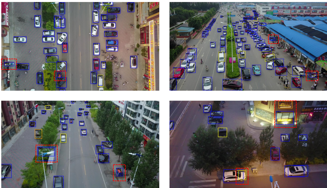
Figure 4: YOLOX predictions on real VisDrone test images. Blue bounding boxes indicate cars, orange indicate trucks, bright yellow indicate vans, and dark yellow indicate buses. Red dashed boxes highlight examples of false positive predictions.
