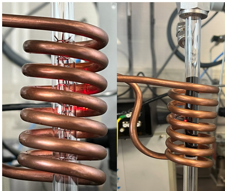
Figure 5. Close-up pictures of the quartz reactor with just the workpiece inside ( left ) and with the catalyst added ( right ) inside the induction heating coil.
