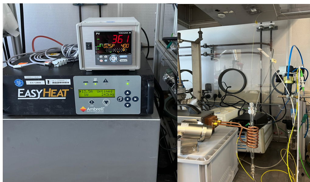
Figure 3. Photo of the induction heating experimental setup.
