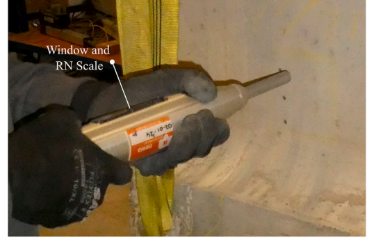
Fig. 2. Rebound hammer device (left) and application on a precast concrete element.
