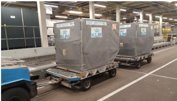
Figure 1: Train of two trailers with Unit Loading Devices (ULD) behind a baggage tug.
