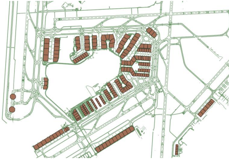
Figure 10: Overview of VOPs and road infrastructure at Schiphol Airport.
