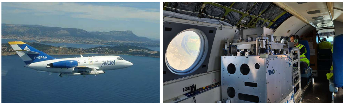
Figure 2. Falcon 20 A/C operated by Avdef (left); OH mass model installed inside A/C cabin for vibration test flight (right).
