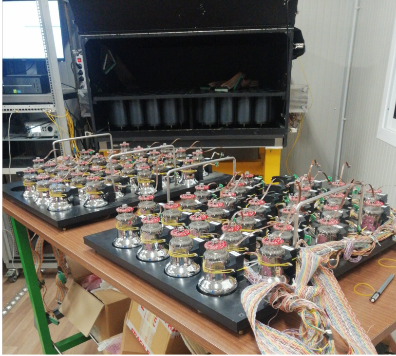
Figure 5. Dark-Box apparatus and two trays of 31 R14374-02 PMTs corresponding to two DOMs. The details can be found in [14].
