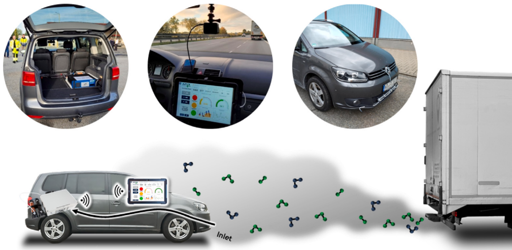
Fig. 1. Setup of Plume Chasing. The tablet is used to display real-time data and is connected to the ICAD instrument via WIFI.
