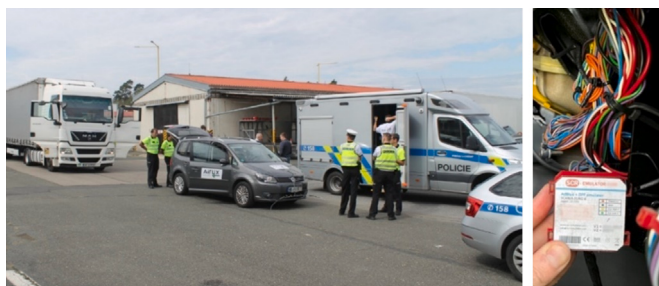
Fig. 8. Inspections of HDVs by Czech police identified as high NO x emitters using the Plume Chasing method (left); example of a commercially available emulator found in the cable tree during the inspection of high NO x emitters (right).
