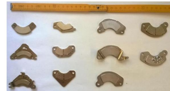
Fig. 3. The examples of magnets assembly of actuator from different hard disk drives (HDDs)
