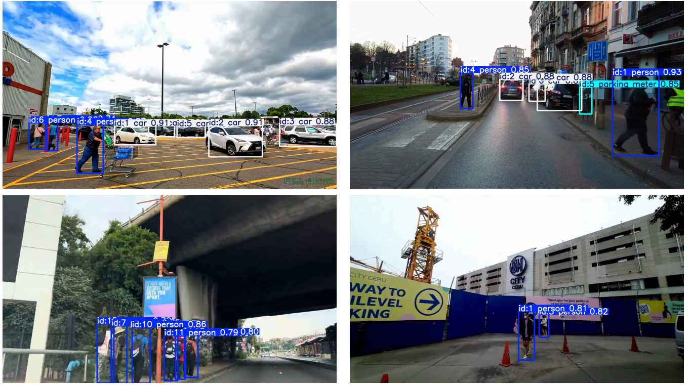
Figure 10: Sample frames illustrating detected pedestrian crossings with YOLOv11x-assigned IDs and confidence values from four selected videos. The top row shows the two slowest detected crossings. Left: the slowest crossing, with the person marked as ID 4 moving at 0.5 m/s (YouTube ID: STbVEZMJdC0); right: the second slowest crossing, with the person marked as ID 4 at 0.5 m/s in Brussels, Belgium (YouTube ID: P00zkZ3_yYY). The bottom row shows the two fastest detected crossings. Left: the fastest crossing, with the person marked as ID 1 at 2.5 m/s in Johannesburg, South Africa (YouTube ID: rnTP1WqduEg); right: the second fastest crossing, with the person marked as ID 1 at 2.5 m/s in Cebu City, Philippines (YouTube ID: Wc6_DYNNzqQ).
