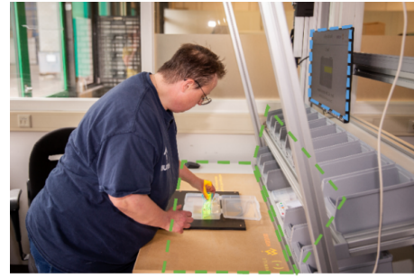
Figure 3: Projection work cel. A projector and time of flight sensor are positioned above the work bench. Information is projected in de green dashed area with additional information on the screen (blue dashed line).
