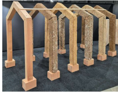
Figure 3. Five decorative portals with biobased fiberboards on a wooden support (left portal); from left to right: Douglas wood support structure, pruning waste, straw, waste wood, hemp shives and bell pepper stems.
