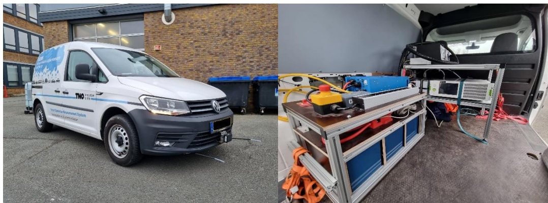
Figure 2.1: TNO plume chase vehicle: Sample inlets and radar on the front bumper, and the licence plate camera behind the window (left). NO x and CO 2 measurement instruments and battery pack in the rear cabin (right).
