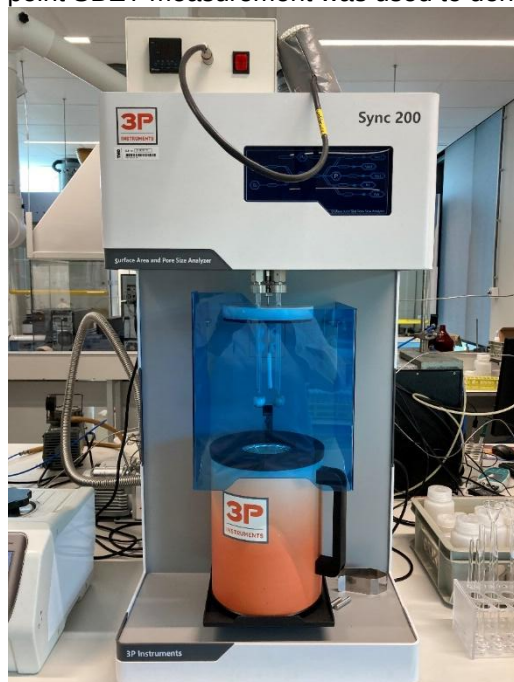
Figure 3 – Photograph of the Sync 200 gas adsorption setup for determining the specific surface area of materials.
