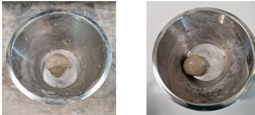
Figure 15 Determining the water demand on the basis of a quick, global consistency method: left mixed ultrafines and right sleeper ultrafines.
