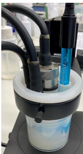
Figure 8 Zeta potential measurement setups showing the set up with four monitoring sensors: zeta potential, conductivity, pH and temperature
