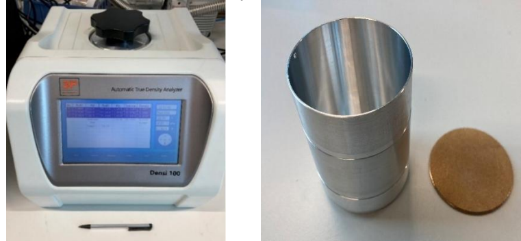
Figure 1 - Photographs of (left) the Densi 100 gas pycnometer set up and (right) the pycnometer itself with end cap.
