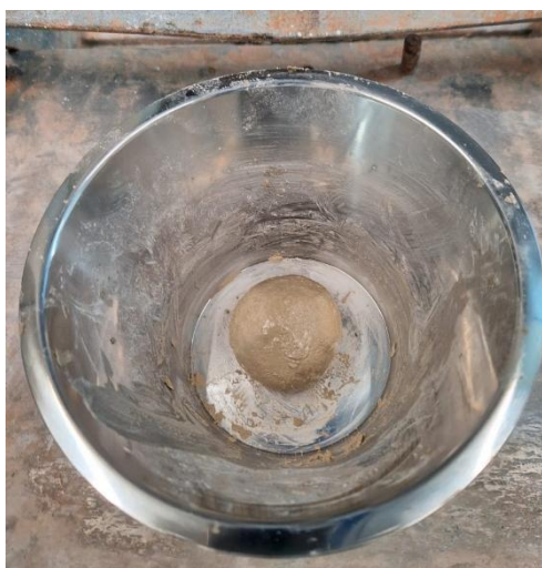
Figure 2.3 Earth dry consistency for CDW_MX during water demand test
