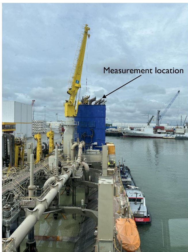
Figure 3.2: Global measurement location (exhaust stack)
